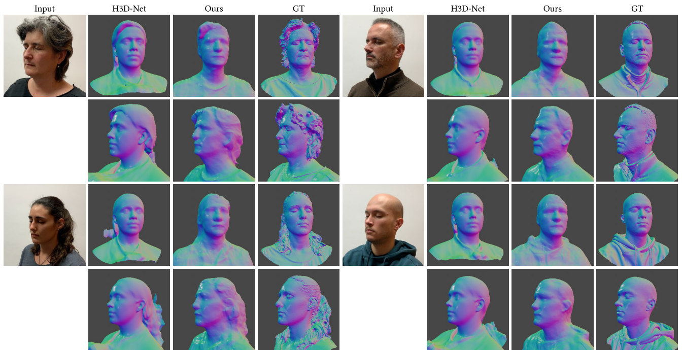
FIGURE 5. Single-view mesh reconstruction on the first four scenes of the H3DS dataset. H3D-Net [4], a method related to ours, was designed for three-view reconstruction but can also be evaluated in the one-shot mode. The H3D-Net system was trained on 10,000 3D scans from the same distribution as these test examples. Our method is trained on a hundred smartphone videos and still matches the quality of H3D-Net, while demonstrating somewhat smaller identity gap and less pronounced regression-to-mean effect.
