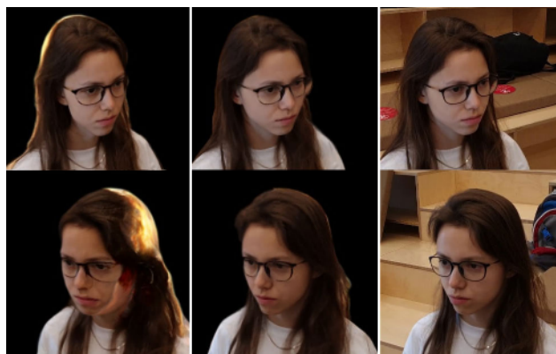
FIGURE 10. A limitation of the underlying architecture of Multi-NeuS: at the second step of fitting, artifacts sometimes reappear in the occluded regions (left column: left cheek and “yellow hair”). Shown are the renders of the control views (top and bottom) for Multi-NeuS fitted to one frontal (left) and two \pm 45^\circ (middle) views next to the ground truth (right). Here we apply our best model on a validation scene from SmartPortraits.
